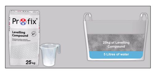
Apply Profix® Levelling Compound to **minimum** 15mm thickness for tiles or engineered wood flooring. Apply Profix® Levelling Compound to **minimum** 18mm thickness for carpet or vinyl flooring.
