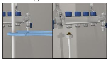
Connect all additional pipe runs to the manifold. Pressure test the system to ensure there are no leaks. Suitable expansion joints should be fitted at all door thresholds.
